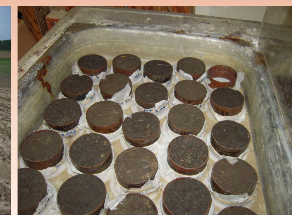
Soil samples on sand table for water retention curve measurements.
