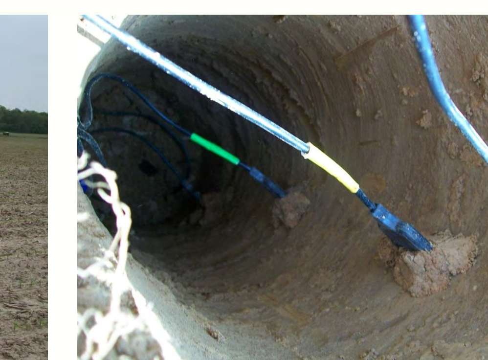
Soil temperature and moisture sensors at respective depths.
