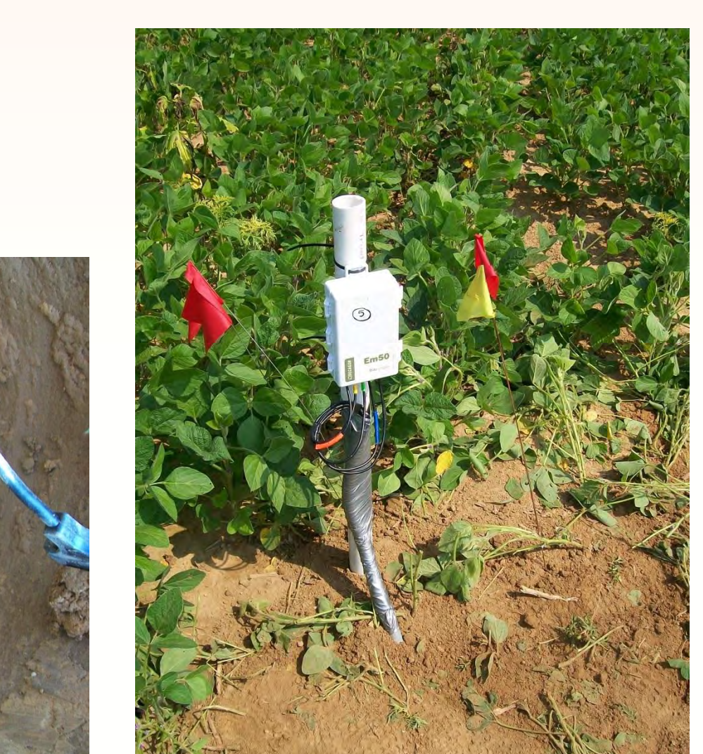
Installed soil temperature and moisture sensors equipped with data logger.
