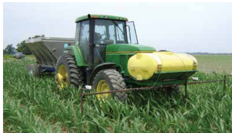
^ Optimal nitrogen fertilizer rate varies widely within a field. Using equipment to sense the nitrogen needs in the corn canopy while applying N fertilizer is a promising approach to diagnose and treat the variation in real time. Two sensors are mounted on either side of the tractor, in front. A computer in the cab reads the sensors, calculates N rate and directs the controller to apply a particular rate of fertilizer.
