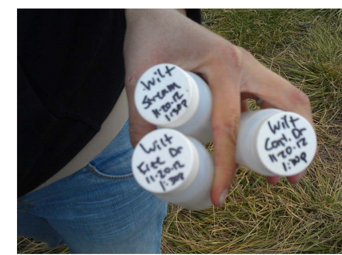
Grab Samples were taken from inside the controlled and conventional drainage structures and were analyzed for dissolved nitrate ( \text{NO}_3^- ) and dissolved phosphate ( \text{PO}_4^{3-} )
