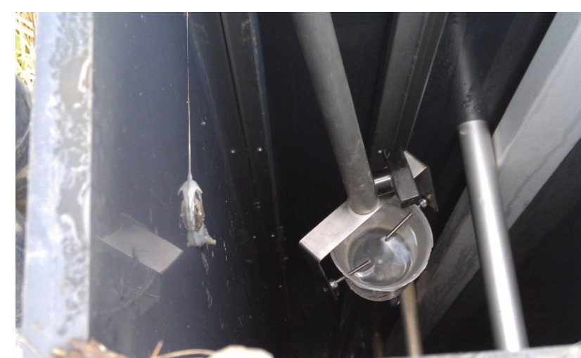
Grab Samples were taken from inside the controlled and conventional drainage structures and were analyzed for dissolved nitrate ( \text{NO}_3^- ) and dissolved phosphate ( \text{PO}_4^{3-} )
