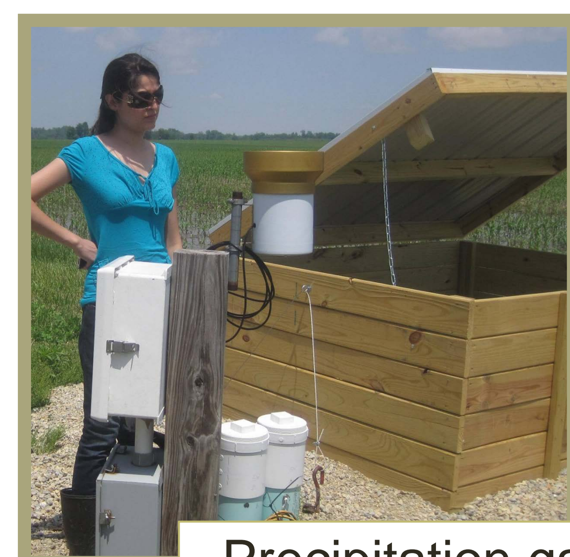
Precipitation gage and data logger with modem
