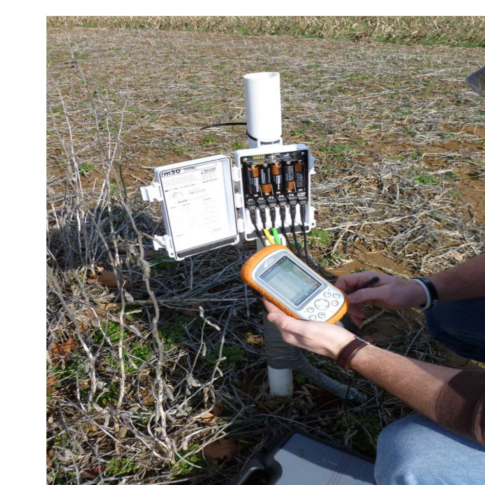
Downloading continuous soil moisture and temperature data to handheld field PC.
